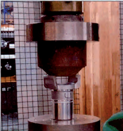
Fig. 1. Cone steel hardness greater than 250 HB 2. body under test 3. Base ground, flat and rigid 4. Force (N) as applied with a maximum speed of 5 mm/s, or in our case a gradual pressing hydraulic force.
