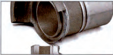
Claw torn broken in snatch test on a couple of sealed Guillemin couplings
