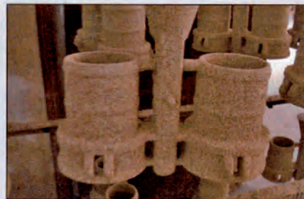
stainless steel in-process sand castings with standard 2-clamp hose shank
